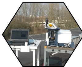
Prototype CHRIS (Compact High-spectral Resolution Infrared Spectrometer).
